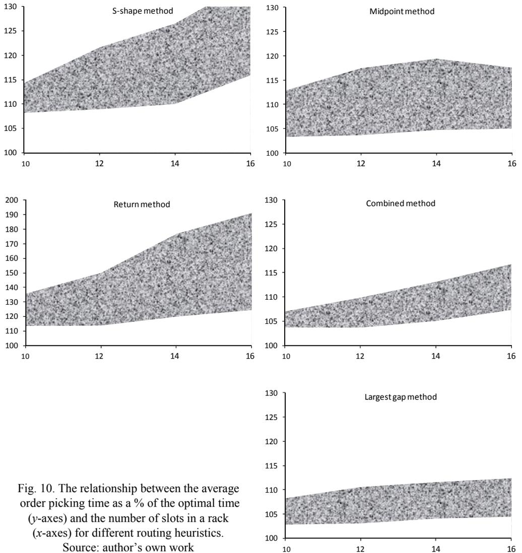
Fig. 10. The relationship between the average order picking time as a % of the optimal time (y-axes) and the number of slots in a rack (x-axes) for different routing heuristics.
