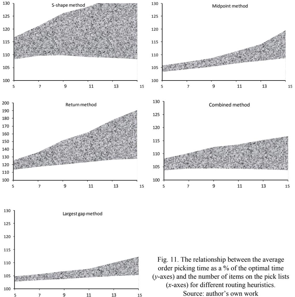
Fig. 11. The relationship between the average order picking time as a % of the optimal time (y-axes) and the number of items on the pick lists (x-axes) for different routing heuristics.
