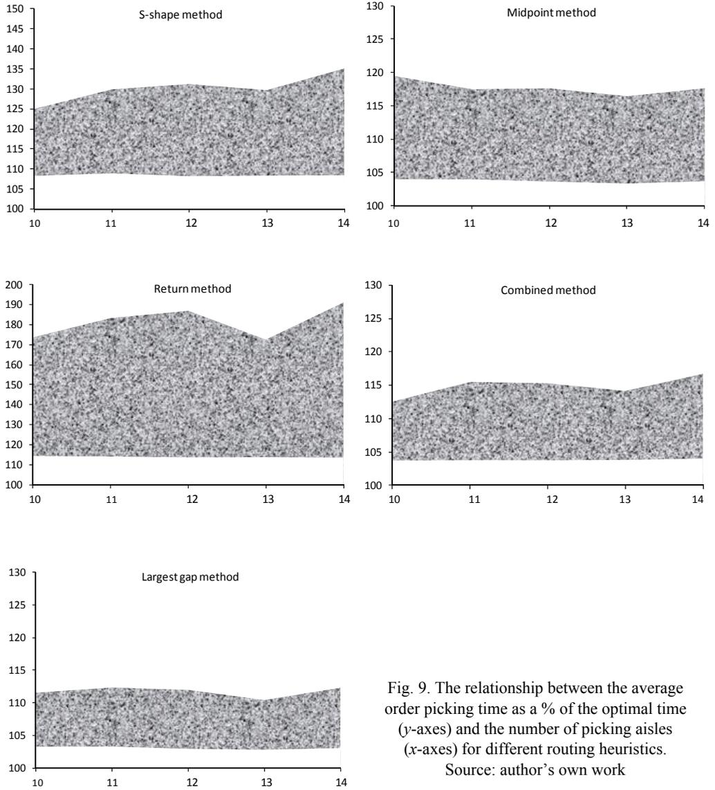
Fig. 9. The relationship between the average order picking time as a % of the optimal time (y-axis) and the number of picking aisles (x-axis) for different routing heuristics.
